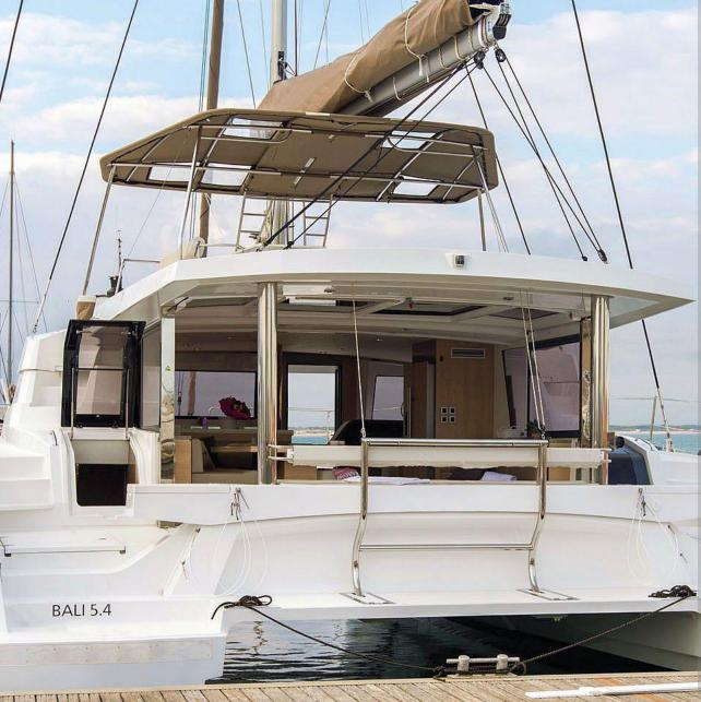
BUILDER CATANA BAL15.4 CONCEPT: Olivie PONCINRTER BUILT 2021 Maximum upwind sail area 202 m<sup>2</sup> / 2,174 sq ft 95 m<sup>2</sup> Fully battened Mainsail in Dacron with 3 reefs 60 m<sup>2</sup> Self-tacking "cross cut" Solent Jib in Dacron ENGINES 2 x 80 hp Yanmar CRUISING SPEED 6.3 KNOTS
